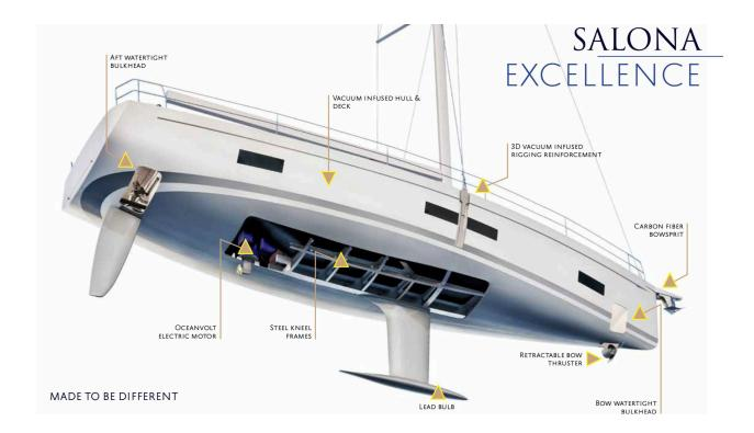
Design is always moving forward and new paradigms allowed by electric propulsion are allowing for many new ideas and innovative solutions. Understanding the needs and numbers is very important, and we will start with power. The old way was **Horse Power (HP)** and now we are talking about **kilowatts (kW)**. HP is a marketing number that is based on the engine's maximum power over time.
